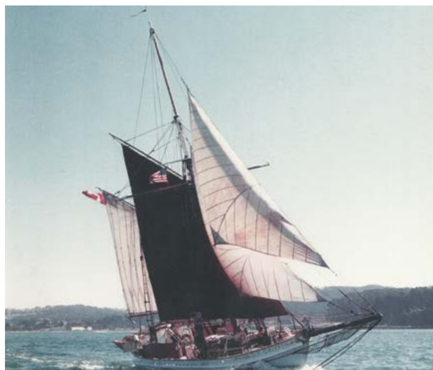
The gaff-rigged ketch, O.R. Griffin , under full sail in a spanking breeze. Photographer unknown.
